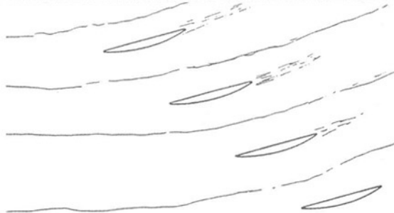
Fig. 15 Photograph and sketch of the smoke flow visualization for \xi = 36.5 deg and \alpha^* = 15 deg
