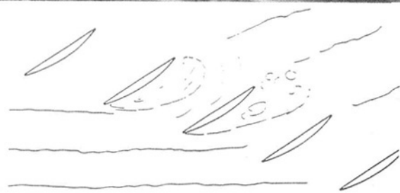
Fig. 17 Photograph and sketch of the smoke flow visualization for \xi = 36.5 deg and \alpha^* = 35 deg
